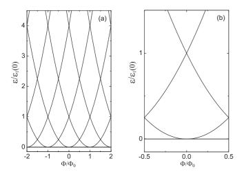
FIG. 1. (a) The energy spectrum of an infinitely narrow quantum ring pierced by a magnetic flux  $\Phi$ . Each parabola corresponds to a particular value of the electron angular momentum *m*. The electron energies  $\varepsilon$  are plotted vs the number of flux quanta  $\Phi/\Phi_0$ . (b) Expanded view on a smaller energy scale.
