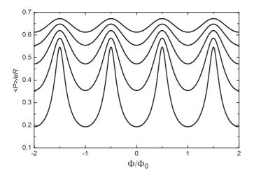
FIG. 5. Magneto-oscillations of the dipole moment of a ring at various magnitudes of the in-plane electric field for  $T = 0.01\varepsilon_1(0)/k_B$ . Different curves correspond to different magnitudes of the electric field in the range from  $E = 0.2\varepsilon_1(0)/eR$  to  $E = 1.0\varepsilon_1(0)/eR$  with the increment  $0.2\varepsilon_1(0)/eR$ . The upper curve corresponds to  $E = 1.0\varepsilon_1(0)/eR$ .
