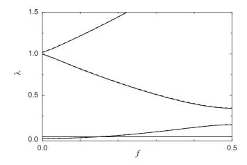
FIG. 8. The normalized energy spectrum as a function of dimensionless parameter f for  $\beta = 0.1$ . Dashed line: the result of analytical solution of the 3 × 3 system. Solid line: the result of numerical diagonalization of the 23 × 23 system. A horizontal line is shown to indicate  $\lambda = 0$  value.
