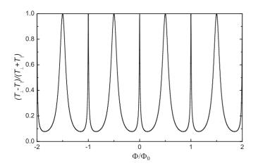
FIG. 7. Magneto-oscillations of the degree of polarization for the transitions between the ground state and the first excited state. Here,  $T_{\parallel}$  and  $T_{\perp}$  are correspondingly the intensities of transitions polarized parallel ( $\mathbf{e} \parallel \mathbf{E}$ ) and perpendicular ( $\mathbf{e} \perp \mathbf{E}$ ) to the direction of the in-plane electric field.
