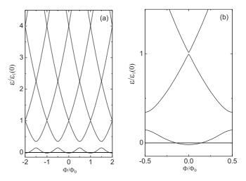
FIG. 2. (a) The energy spectrum of an infinitely narrow quantum ring of radius *R* pierced by a magnetic flux  $\Phi$  and subjected to an in-plane electric field  $E = 0.2\varepsilon_1(0)/eR$ . The electron energies  $\varepsilon$  are plotted vs the number of flux quanta  $\Phi/\Phi_0$ . (b) Expanded view on a smaller energy scale.
