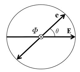
FIG. 6. Relative directions of the external electric field **E** and the projection **e** of the THz radiation polarization vector onto the quantum ring's plane.
