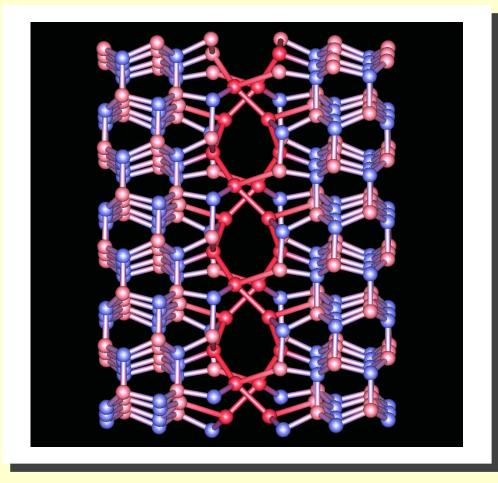
Gallium-core model of a threading screw dislocation in wurtzite gallium nitride radiated at low temperatures might contain substantial amounts of energy which could pose a problem if released inadvertantly.
