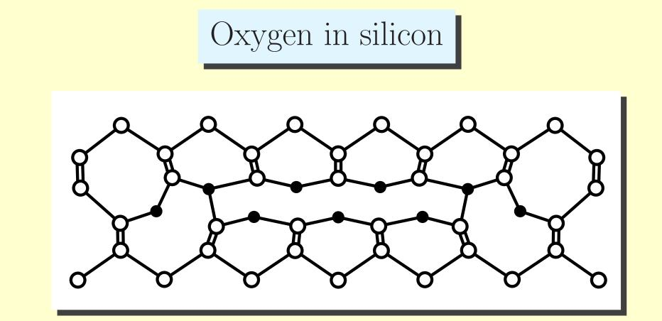
A collaboration with the experimental group at Lund (Sweden) into the nature of the **thermal donor** defect in silicon has lead to a model of the donor, shown above  $(\bigcirc - \text{Si}, \bullet - \bigcirc)$ , which agrees with their experimental results.
