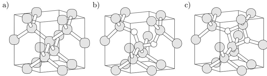
**Figure 6.4:** The structures of the oxygen pair. The stable form of the pair in the neutral and single positive charge states is labelled  $O_{2i}^{st}$  (structure *b* above).  $O_{2i}^{sq}$  (structure *c* above) is the stable form of the pair in the double positive charge state. A piece of equivalent bulk material (structure *c*) is also shown. As before, grey balls represent Si and small white ones represent O.
