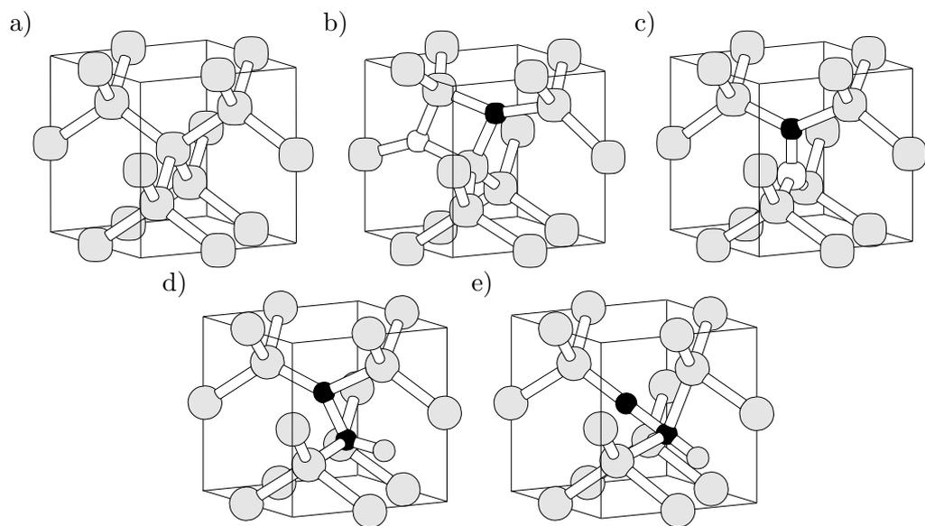
**Figure 5.1:** The calculated structures of the boron-impurity complexes assigned to the experimentally observed levels. (a) a piece of bulk Si to aid the reader, (b)  $B_iO_i$ , (c)  $B_iC_s$ , (d)  $B_iB_sH$  in the neutral and negative charge state, (e)  $B_iB_sH$  in the positive charge state. Large grey balls represent Si, small grey are H, small black are B, small white are O and the larger white ones are C.
