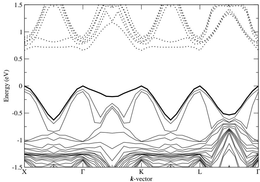
**Figure 6.7:** The Kohn-Sham bandstructure of  $O_{2i}^{st}$ . In the neutral charge state solid lines are filled levels and dotted lines represent unoccupied levels. It is suggested that the highest occupied level (shown as a heavy line) may be a donor (0/+) level of  $O_{2i}$ .
