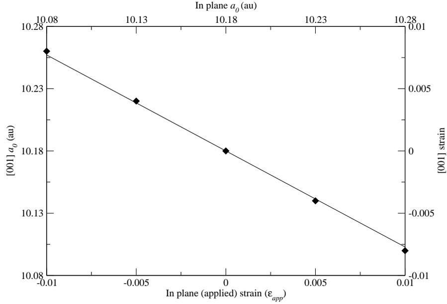
**Figure 7.1:** The variation of relaxed [001] lattice constant with biaxial-strain. Data points are the calculated values while the line is a plot of the equation  $\epsilon_{rel} = -2(C_{12}/C_{11})\epsilon_{app}$  given by elasticity theory. The calculation was performed in supercells of 64 atoms.
