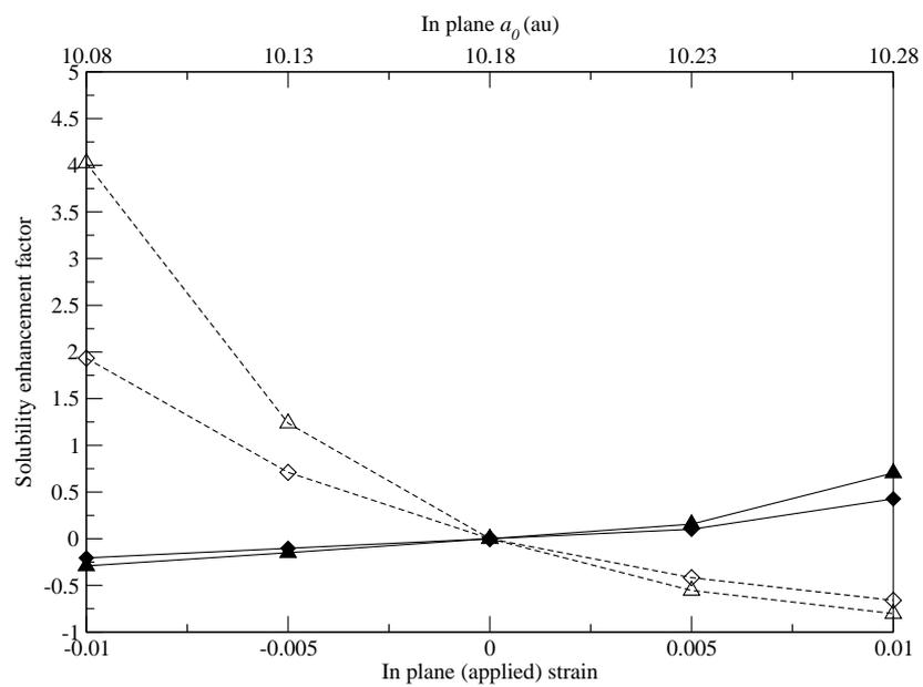
**Figure 7.8:** The enhancement to the equilibrium solubility of arsenic with strain for two different temperatures (triangles correspond to 800 K and diamonds correspond to 1200 K). To illustrate the influence of the change in Fermi-energy the enhancement is shown for a Fermi-energy set to be constant with strain (dashed lines and empty symbols) and for the value of  $E_F$  calculated as a function of strain (solid lines and filled symbols).
