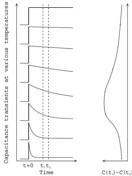
**Figure 2.4:** The double boxcar technique for analysing capacitance transients, introduced by Lang. The rate window is defined by  $t_1$  and  $t_2$ , the times at which the capacitance is measured to give  $\Delta C$ , plotted on the right hand side.
