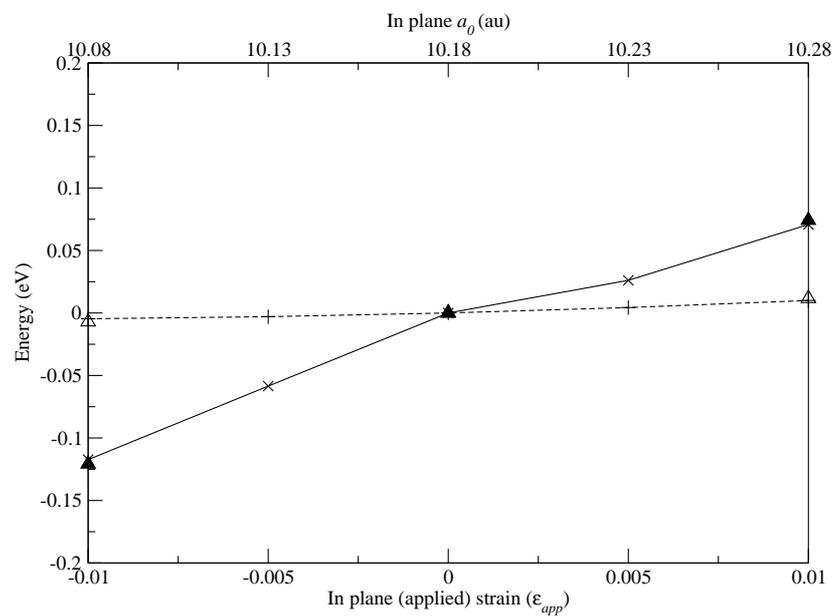
**Figure 7.5:** The variation of formation energy and total energy of substitutional boron with biaxial strain. Pluses joined by a dashed line and crosses joined by a solid line show values calculated using 64 atom supercells for the total energy and formation energy respectively. Empty triangles and filled triangles show the values of the total energy and formation energy respectively calculated with 216 atom supercells to demonstrate convergence.
