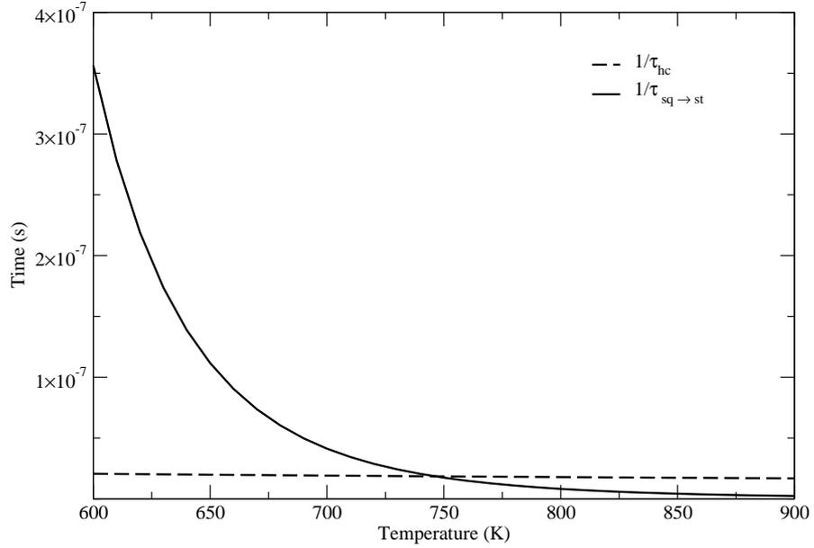
**Figure 6.2:** The time taken for  $B_sO_{2i}^{0sq}$  to capture a hole ( $1/\tau_{hc}$ ) and the time taken for  $B_sO_{2i}^{0sq}$  to be converted to the stable form in the neutral charge state,  $B_sO_{2i}^{0st}$  ( $1/\tau_{sq \rightarrow st}$ ). Note that at room temperature hole capture will take place long before  $B_sO_{2i}$  is able to reconfigure.
