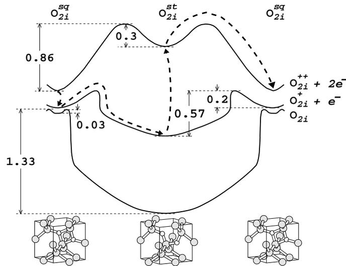
**Figure 6.5:** A configuration coordinate diagram for the oxygen pair. Arrows show the proposed thermally assisted Bourgoin diffusion mechanism with a thermal barrier of 0.3 eV.  $O_{2i}^{++sq}$  at *A* first captures a photo-generated or injected electron and, after overcoming a 0.2 eV barrier, changes its configuration to  $O_{2i}^{+st}$ . It then traps a hole becoming  $O_{2i}^{++st}$ , and executes a diffusion jump to  $O_{2i}^{++sq}$  at *B* after overcoming a thermal barrier of 0.3 eV.
