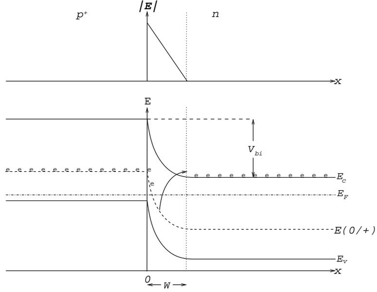
**Figure 2.1:** A  $p^+n$  Schottky barrier diode showing the associated band bending. Above the band structure is a plot of the electric field caused by the band bending on the same  $x$ -axis. The  $n$ -type region has  $x > 0$  while  $x < 0$  is  $p^+$ -type.
