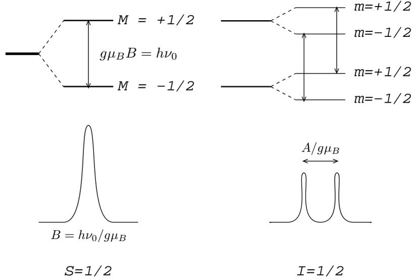
**Figure 2.6:** The allowed EPR transitions for a system with electron spin  $S = 1/2$  (left) and with nuclear spin  $I = 1/2$  (right). The curves show the resonance as a function of magnetic field while the lines above show the transitions between levels that have been split due to the Zeeman effect. For ENDOR there are also transitions allowed for  $\Delta M = 0$ ,  $\Delta m = 1$ .
