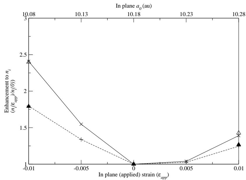
**Figure 7.3:**  $n_i(\epsilon_{app})/n_i(0)$  calculated using 64 and 216 atom supercells for two different temperatures. The crosses joined by a solid line and the pluses joined by a dashed line are values calculated using 64 atom supercells for  $T = 800$  K and  $T = 1200$  K respectively. Empty and filled triangles are the values calculated in 216 atom supercells for  $T = 800$  K and  $T = 1200$  K respectively demonstrating the convergence with respect to cell size.
