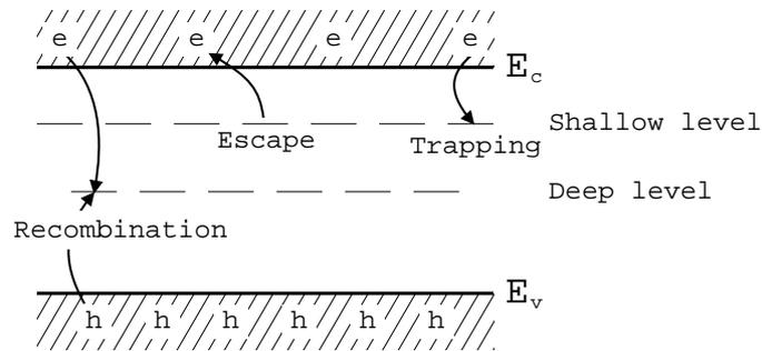
**Figure 2.9:** The trapping model of [Hornbeck and Haynes \(1955\)](#) for a  $p$ -type semiconductor. Recombination is considered to occur at a single deep level. A second, shallow level is able to trap carriers which may later be released.
