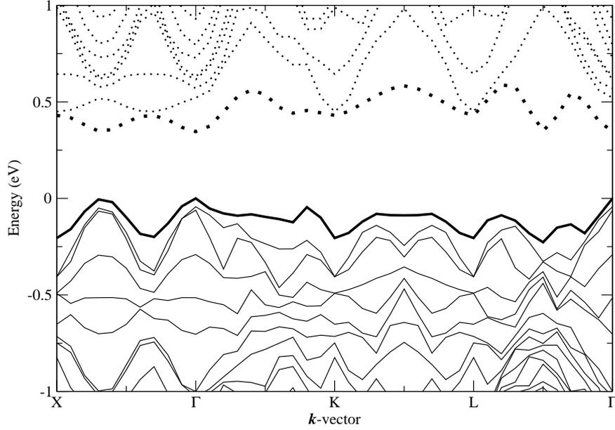
**Figure 4.3:** The calculated Kohn-Sham band-structure of  $B_2I_3^Y$  in a 96 atom supercell. Dotted lines indicate levels which are empty while solid lines indicate levels which are filled in the neutral charge state. Note the shallow level present at each band edge indicated by heavy lines.
