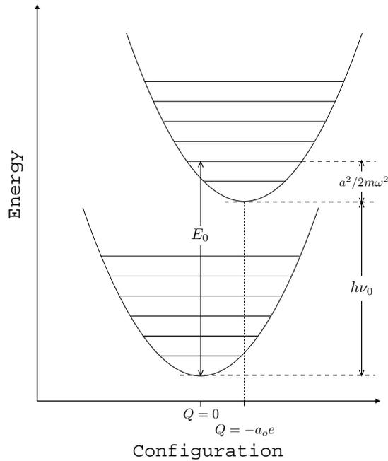
**Figure 2.5:** A configuration coordinate diagram showing the ground and excited states of a PL transition. The zero phonon line has energy  $h\nu_0$ .
