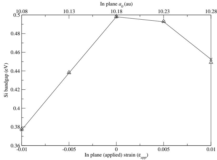
**Figure 7.4:** The variation in size of the Kohn-Sham band-gap of silicon with biaxial strain. The solid line with crosses shows values calculated using 64 atom supercells while triangles show the values calculated using 216 atom supercells.
