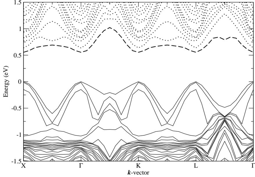
**Figure 6.3:** The Kohn-Sham band-structure of  $B_sO_{2i}^{sq}$  calculated in a 64 atom supercell. Dotted lines represent conduction band levels, solid lines indicate valence band levels and the dashed line represents the donor (0/+) level.
