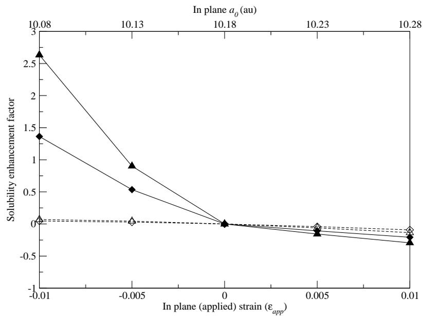
**Figure 7.6:** The enhancement to the equilibrium solubility of boron with biaxial strain for two different temperatures (triangles correspond to 800 K and diamonds correspond to 1200 K). To illustrate the influence of the change in Fermi-energy the enhancement is shown for a Fermi-energy set to be constant with strain (dashed lines and empty symbols) and for the value of  $E_F$  calculated as a function of strain (solid lines and filled symbols).
