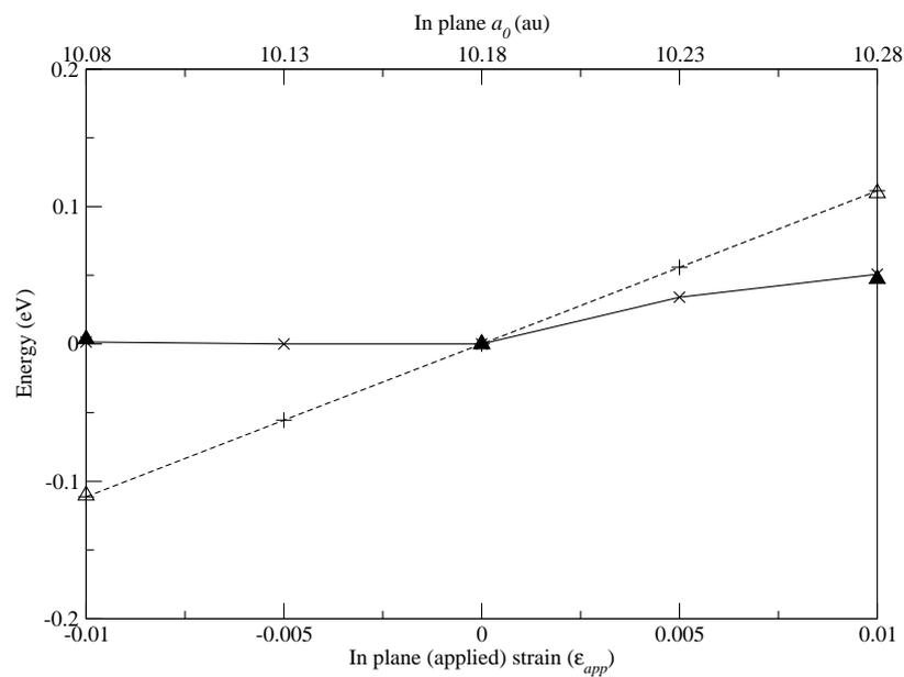
**Figure 7.7:** The variation of formation energy and total energy of substitutional arsenic with biaxial strain. Pluses joined by a dashed line and crosses joined by a solid line show values calculated using 64 atom supercells for the total energy and formation energy respectively. Empty triangles and filled triangles show the values of the total energy and formation energy respectively calculated with 216 atom supercells to demonstrate convergence.
