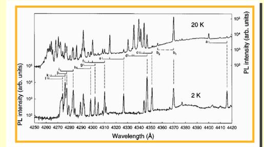
Silicon carbide is being developed as a **high temperature electronics material**. An unusual feature is the creation of defects giving 40 luminescent lines within a 0.1 eV interval (above) when the material is irradiated. Collaborative work with Bristol University has led to a model for these centres based on an anti-site defect where a silicon atom occupies a carbon site.
