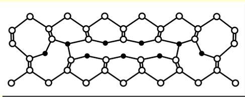
A collaboration with the experimental group at Lund (Sweden) into the nature of the **thermal donor** defect in silicon has led to a model of the donor, shown above (○ - Si, ● - O), which agrees with their experimental results.
