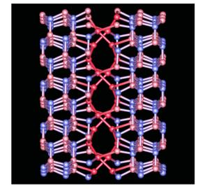
Gallium-core model of a threading screw dislocation in wurtzite gallium nitride
