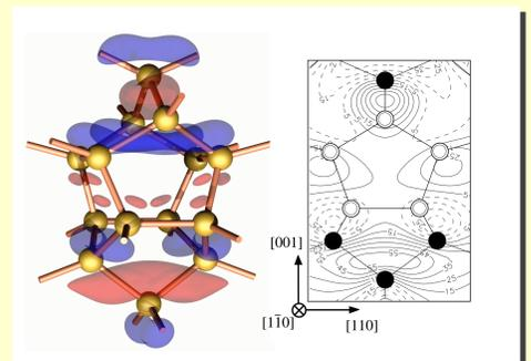
There is intense interest in the properties of multi-interstitial centres in silicon formed after **ion-implantation**. We have recently succeeded in identifying two such aggregates, one of which is shown above, giving rise to prominent optical emissions. The work is carried out in association with experimental groups at King's College London and Brunel University.
