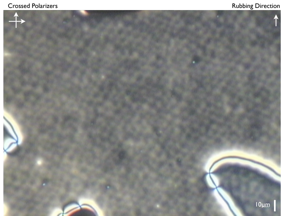
Figure 3.10: Polarizing microscopy image of a hybrid aligned cell in the nematic phase following repeated cooling and heating through the nematic–smectic transition. The intensity of illumination is high revealing a “surface memory” of the low temperature “fan” structure even though the liquid crystal is here in the nematic phase as may be seen from the presence of disclination lines.
