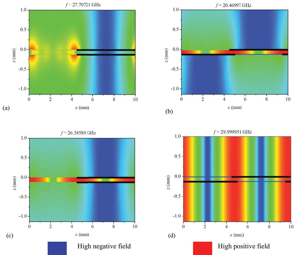
FIG. 5. (Color online) Complex magnitude  $\vec{E}$  field plots in the  $XZ$  plane for a double-mesh-layer system of pitch  $d = 10$  mm, hole side length  $a = 4.5$  mm, and mesh separation  $g = 0.1$  mm at (a) 27.7 GHz with misalignment  $b = 0$  mm; (b) 20.4 GHz with misalignment  $b = 5$  mm; (c) 25.5 GHz with misalignment  $b = 0$  mm; and (d) 29.9 GHz with misalignment  $b = 5$  mm. The metal meshes are represented by thick black lines.
