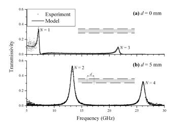
FIG. 3. Experimental frequency-dependent transmissivity data from (a) a structure whose slits on either side of the core are directly opposite each other (d = 0 mm), and (b) a structure with  $d = \lambda_g/2 = 5$  mm. Also shown are the numerically modeled results. Radiation is normally incident ( $\theta = 0^\circ$ ) and detected, and the sample is orientated so that the slit direction is perpendicular to the electric field vector.
