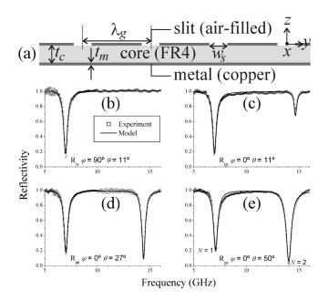
FIG. 1. Experimental reflectivity spectra and the numerically modeled results from the structure illustrated schematically in (a). (b) The  $R_{ss}$  response of the structure when orientated with the slit direction parallel to the plane of incidence ( $\varphi = 90^{\circ}$ ). (c)–(e) The  $R_{pp}$  response with  $\varphi = 0^{\circ}$  at three different angles of incidence. The change in noise at 10 GHz corresponds to a switch in the set of waveguides and horn antennas used.
