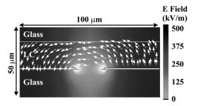
FIG. 6. Modeled electric field for a 25  $V_{pp}$  in-plane potential difference applied across a 25  $\mu$ m gap. The gray scale indicates the electric field intensity and the arrows indicate the corresponding field lines.
