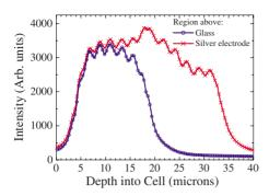
FIG. 5. (Color online) Comparison of recorded fluorescence intensity (arbitrary units) versus depth into the sample for regions above the silver electrode and glass electrode gap.
