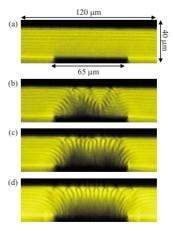
FIG. 4. (Color online) Cross-section images from a MLC-6608 liquid crystal cell showing the fluorescence intensity as a function of position at applied peak-to-peak voltages of (a) 0, (b) 40, (c) 60, and (d)  $100~\rm V$ .
