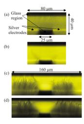
FIG. 3. (Color online) Cross-section images from a ZLI-2293 liquid crystal cell showing the fluorescence intensity as a function of position at applied peak-to-peak voltages of (a) 0, (b) 15, (c) 25, and (d) 50 V.
