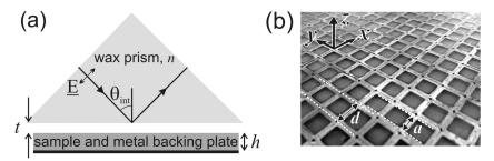
Fig. 1. (a) Schematic of the experimental set-up. (b) Photograph of sample surface and experimental coordinate system, where a = 6.96 mm and d = 9.53 mm.
