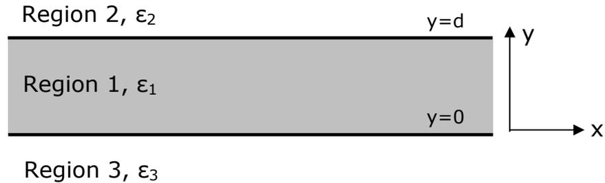
Figure 2.5 an asymmetric planar slab waveguide structure.
