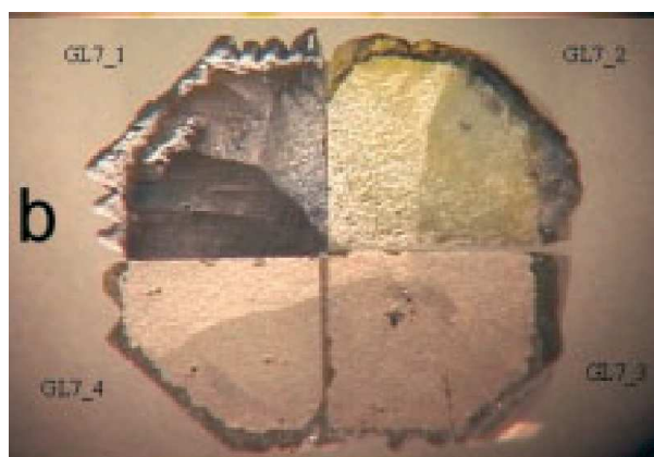
Figure 1.11: The removal of brown colour by HPHT treatment, taken from Charles et al. [34]. Proceeding clockwise from the top left are: (a) The as-grown diamond (b) Treated at 1900° C (c) Treated at 2200° C and (d) Treated at 2200° C for a longer time.
